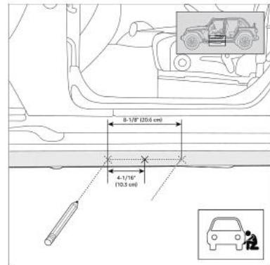
**3** Drill a 3/8" hole on these points. Before drilling make sure you center the 3/8" drill bit on the flange, use a center punch and 1/8" drill bit to drill a pilot hole for best results.
