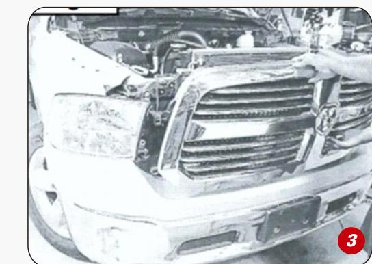
(3)Firmly grab and pull factory grille off vehicle. Set factory grille aside for later use.
