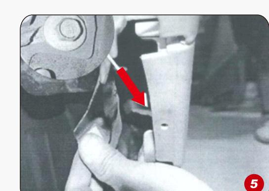
(5)Pull back inner fender and upper trim piece to allow access behind the inner fender to remove one factory bolt, securing the headlight trim piece onto vehicle. Using a 10mm socket remove bolt. Set aside for later use. Repeat step 4-5 for other side.
