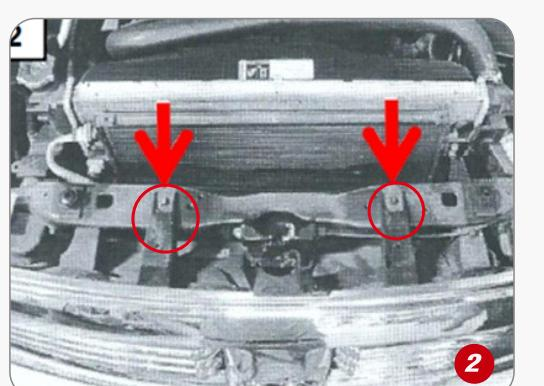
(2)Using a 10mm socket locate and remove 4 factory hex head bolts securing the grille onto the vehicle. Set hardware aside for later use.
