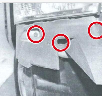
(9)Using a 10mm socket locate and remove 3 factory bolts holding the center plastic onto vehicle. Discard plastic center. Repeat step for other side.
