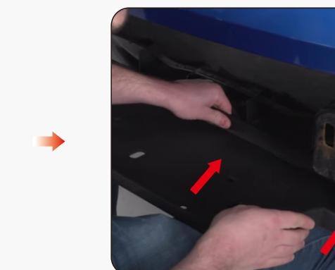
(1)Place Factory Hood release bracket back into the truck. Line up the holes in the Bumper Cap with the holes in the Hood release bracket.
