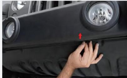
**2** Remove the factory fog light connections by pushing the tab in on the brown connector and gently pulling out.
