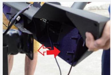
**8** Each of the 3 pre-installed bolts will attach with a flat washer, lock washer and nut. All 8 bolts connections will be tightened as shown partially completed in the following pictures.
