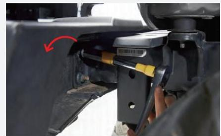
**4** If you are installing a winch, remove the frame cover. This requires removing the center pin from the two clips, then pulling the clips out.or some prefer to leave it on if not running a winch, with applicable bumpers.
