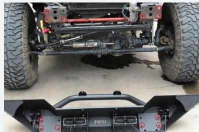
**7** Now it's time to bolt the bumper up into place. Ideally, a second person would help hold the bumper into place.
