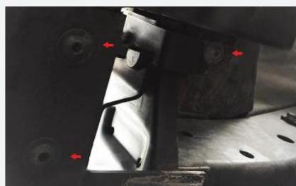
**3** Remove 18mm bottom side bolt on the driver and passenger side of the bumper.
