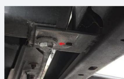
**4** Remove the 2 back side 18mm bolts on drive and passenger side of the bumper.
