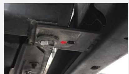
**2** Remove the 3 bolts on each side of the bottom side of the bumper.
