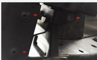
**3** Remove 18mm bottom side bolt on the driver and passenger side of the bumper.
