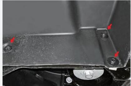
**3** Once the splash shields are removed, locate and remove the (2) 16mm bolts securing the splash shield brackets to the bumper. Bumper will now be loose.
