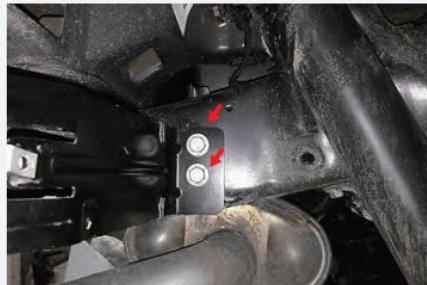
**4** If equipped, remove the four 21 MM bolts holding the factory tow hook to the frame.
