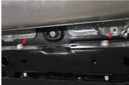
**2** Locate and remove the (3) 8mm screws securing the splash shield to the bumper. Remove splash shield.
