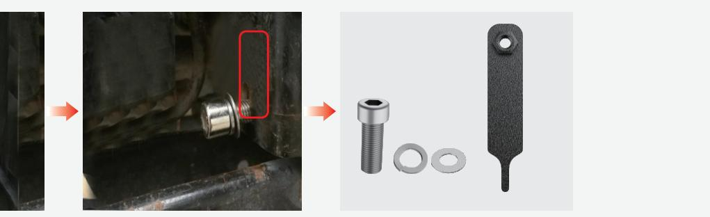
2 Install the PART "B" on it, and tighten the PART "H" with 10mm L type wrench. As shown below. (Please browse the note before step2, the steps are slightly different depending on the position of the carbon cylinder)
