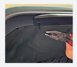
Cut off the redundant rivets and complete the installation.
