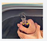
Align the wheel eye brow with the hole position, and nail the rivet.
