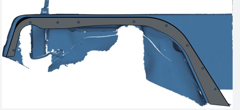
(3) Secure the front fender flare on body panel with (9) M5x15 drilling screws.
