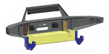
(2) Line up the holes in bumper guard with the holes in winch mounting plate and bumper. Place a supplied M6\*20 hexagon bolt (K1) with M6 flat washer (K2) through the hole in the bumper guard and through the hole in the bumper. Place a supplied M6 split washer (K3) at the end of bolt. Tighten down bolt. Repeat step for remaining bolt.
