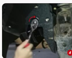
5 Step5 Install the 2 "PART G" on the bumper.
