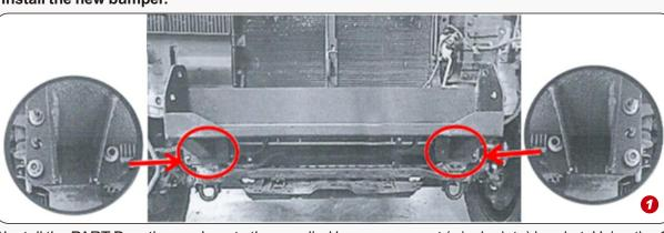
(1)Install the PART D on the car. Locate the supplied bumper support (winch plate) bracket. Using the OEM nuts from the removal process mount the PART D to the vehicle and tighten down.
