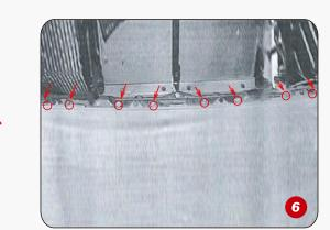
(6)Using a 10mm socket remove the 8 bolts from the center portion of the bumper cap.
