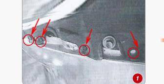
(1)While underneath the vehicle, locate and remove the four 8mm bolts that hold the plastic guard on each side of the bumper to gain access to the bolts attaching the bumper to the frame.
