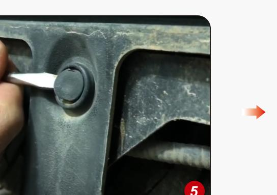
(5)Unclip plastic clips that are holding the plastic step to the top of the bumper.
