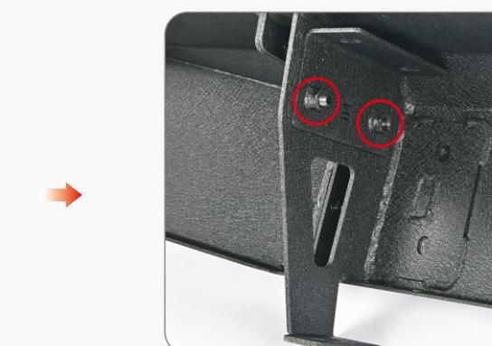
(2)Attach the new bumper, using with 4 of E1, E2&E4.
