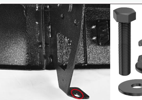
(3)Fix bumper, using with 2 of F1, F2, F4& 8 of F3.
