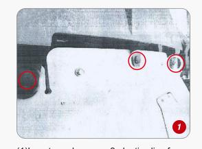
(1)Locate and remove 3 plastic clips from skid plate under vehicle
