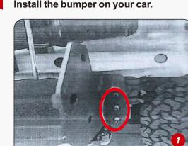
(1)Locate the PART D and place on vehicle frame. Line up the holes in PART D with bolts from frame and using OEM hardware attach bracket.
