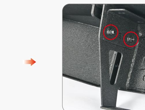
(2)Attach the new bumper, using with 4 of E1, E2&E4.
