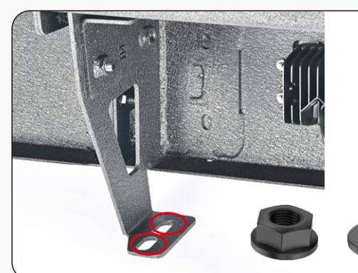
(3)Fix bumper, using with 4 of F1, F2, F4& 8 of F3.
