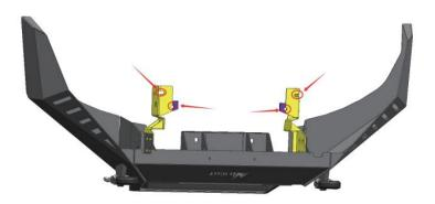
(2) Place supplied M8\*20 hex head bolt (H1) with M8\*16 flat washer (H3) through the hole in the side of the bracket. Place a M8 flat washer (H3) and a M8 split washer (H4) at the end of bolt. Start a supplied M8 hex head nut (H2) at the end of bolt. Tighten down using a socket. Repeat step for remaining bolt.
