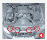
(4) Using a # 2philip's head screw driver locate and remove 4 factory screws holding the factory grille onto vehicle.
