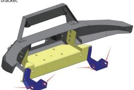
(2) Line up the holes in the winch mounting plate (E) with the holes in the mounting bracket (D). Place supplied M12\*35 hex head bolt (I1) with M12 flat washer (I3) through the hole in the mounting bracket (D). Place a M12 flat washer and a M12 split washer (I4) at the end of bolt. Start a supplied M12 hex head nut (I2) at the end of bolt. Tighten down bolt. Repeat step for remaining bolt.
