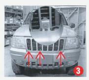
(3)Using a # 2philip's head screw driver locate and remove 3 factory screws holding the factory grille onto vehicle.
