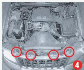
(4) Using a # 2 philip's head screw driver locate and remove 4 factory screws holding the factory grille onto vehicle.
