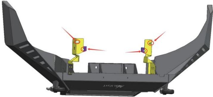
(2) Place supplied M8\*20 hex head bolt (H1) with M8\*16 flat washer (H3) through the hole in the side of the bracket. Place a M8 flat washer (H3) and a M8 split washer (H4) at the end of bolt. Start a supplied M8 hex head nut (H2) at the end of bolt. Tighten down using a socket. Repeat step for remaining bolt.
