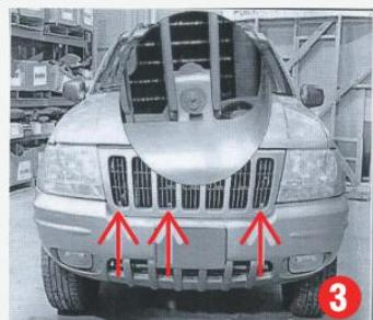
(3) Using a # 2 philip's head screw driver locate and remove 3 factory screws holding the factory grille onto vehicle.
