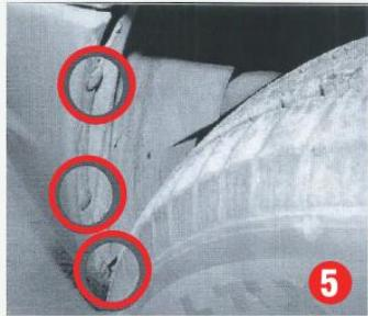
(5) Looking inside the vehicle wheel well locate and remove 3 factory clips holding the bumper onto the vehicle using a plastic removal tool. Repeat step for other side.
