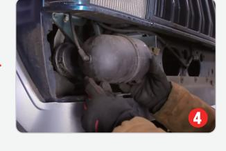
(4) Remove vacuum canister from bumper and set it aside for later use.
