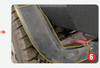
(5) In order to facilitate product installation and product better fit. Remove the original front baffle. Cut off the excess on both sides. As the picture shown. (Note: Only 96 and earlier require fender trimming)
