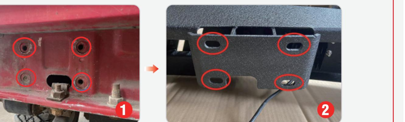
(2) With help from an assistant place bumper onto vehicle. Place a supplied M12\*30 hex head bolt (D1) with M12\*30 flat washer (D2) through the hole in the bumper and through the holes in the mounting bracket (B). Place a M12\*30 flat washer and M12 split washer (D4) at the end of bolt. Start a M12 hex head nut (D3) at the end of bolt. Tighten down using a socket. Repeat step for remaining bolt.
