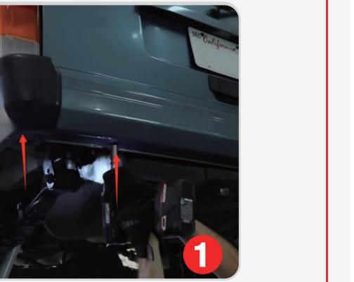
(2) Locate and remove 8 factory bolts holding the bumper onto vehicle. With help from assistant remove factory bumper from vehicle.
