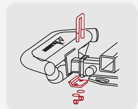
**1** Insert the hitch step into the hitch receiver
