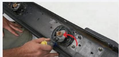
**5** Install the factory fog lights into the openings in the back of the new bumper using the factory screws. Ensure the lights are centered in the housing before tightening all bolts/nuts.
