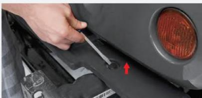
**4** Remove the factory fog lights from the bumper for re-use on your new bumper by removing the 4 screws holding each one in place.
