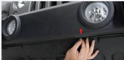
**2** Next, unplug the factory fog lights and loosen the (8) 19mm nuts holding the front bumper to the support beam of the vehicle. Remove the bumper completely.
